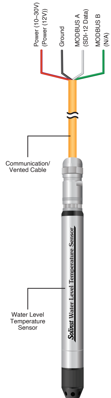
MODBUS Wiring Overview (SDI-12 in Brackets)
